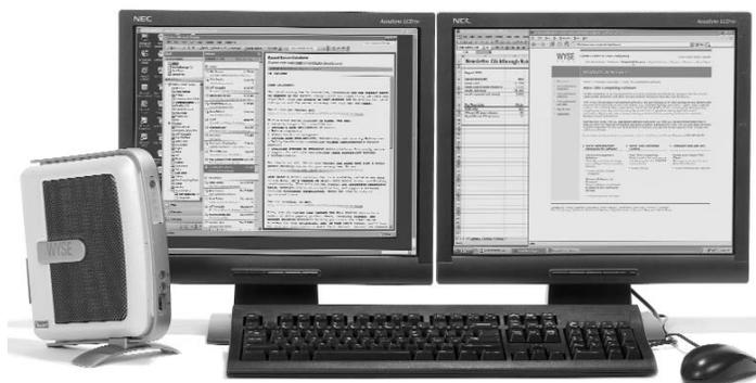
The V-Class Dual-Video thin computer includes a powerful CPU; dual-video support (with purchase of optional monitor splitter cable); 128MB Flash, 256MB DDR RAM; a CardBus/PCMCIA slot; plus serial, parallel, and USB ports. It can sit on a desk in vertical or horizontal position, or be mounted to a wall, desk, or in any space-constrained environment via its monorail mounting system
